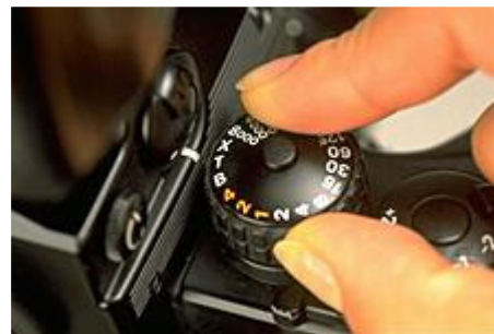
(Photo 0..) In principle, the speedlight should be used at a shutter speed faster than "X"-speed
